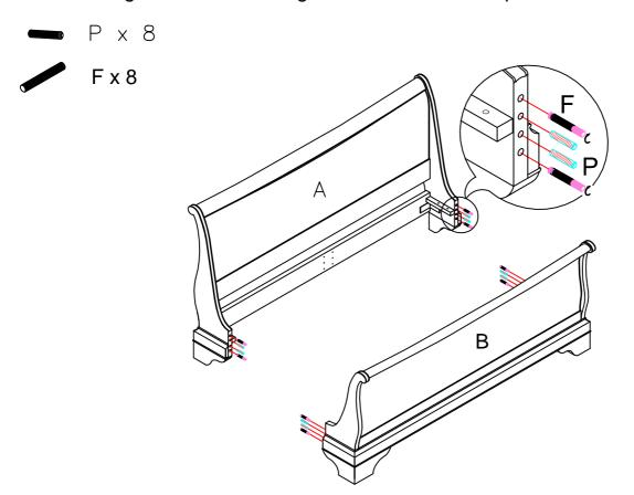
Step ② -Locate the side rails (C) onto the dowels (P) and threads (F) protruding from the headboard (A) and footboard (B). Locate the washer (H & I) and nut (J) onto the threads (F) and secure by hand at first. Tighten using the open ended spanner (G) (provided).
